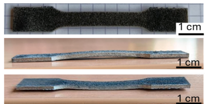
Fig. 5. Distortion of a tensile specimen observed after a heat treatment at 580 °C.
